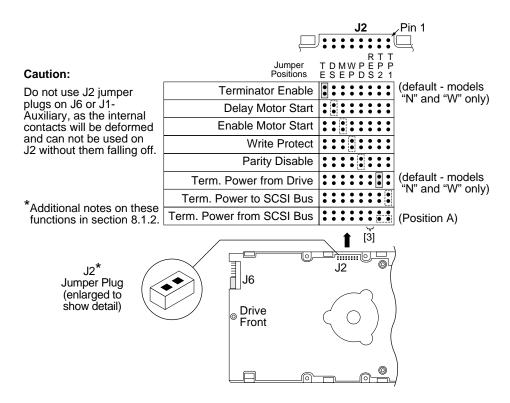
Figure 12. Barracuda 4XL family drive option select header for models "N," "W," and "WD"
