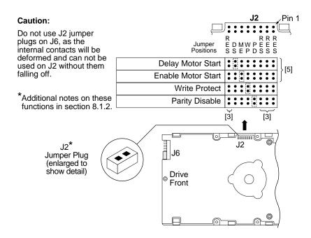
Figure 13. Barracuda 4XL family drive option select header for models "WC" and "DC"
