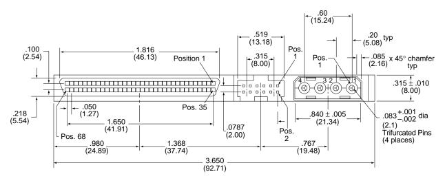
Figure 20. Non-shielded 68 pin SCSI device connector used on "W" and "WD" model drives
