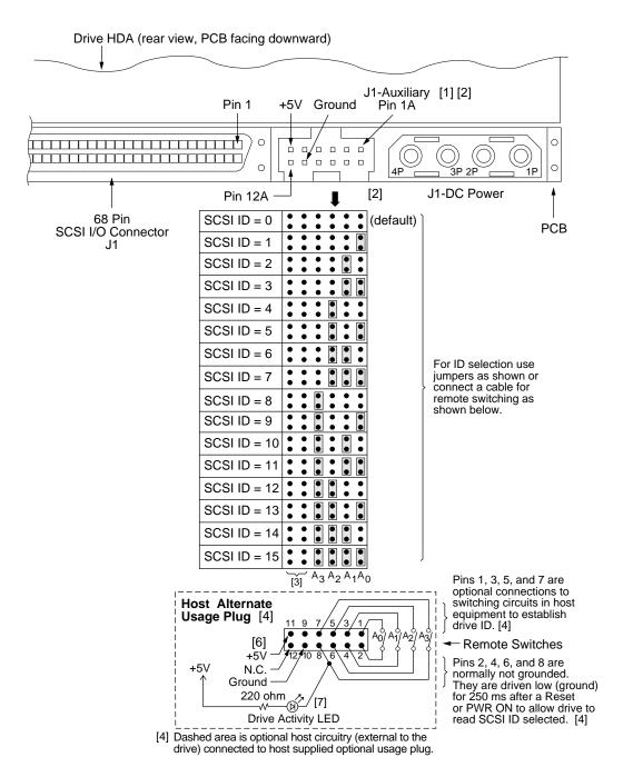
Figure 11. Barracuda 4XL family drive ID select header J1-auxiliary for models "W" and "WD" (J1-Auxiliary Pins 1A - 12A)
