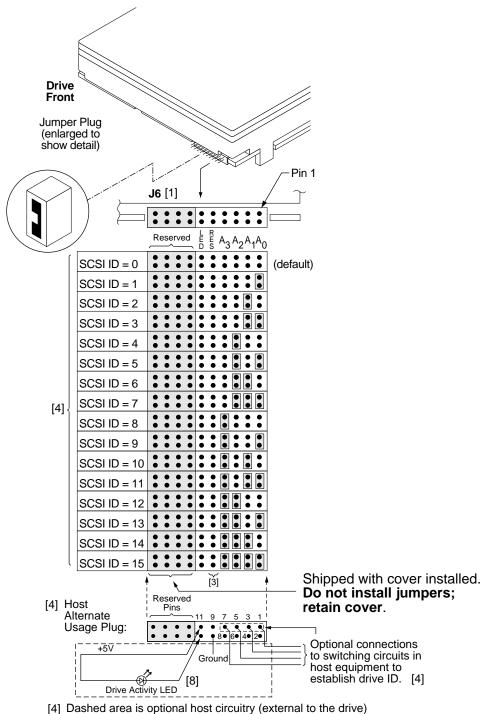
connected to host supplied optional usage plug. **Do not connect anything to pins 13-20.**
