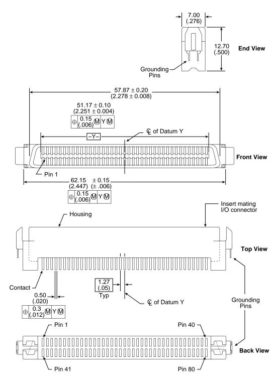
Figure 21. Non-shielded 80 pin SCSI "SCA-2" connector, used on "WC" and "DC" model drives
