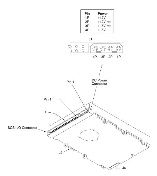
Figure 15. Physical interface for "N" model drives
