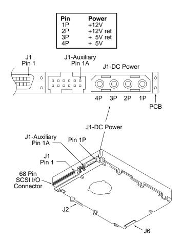
Figure 16. Physical interface for "W" and "WD" model drives
