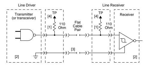
Figure 22. Single-ended transmitters and receivers
