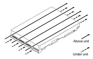
Note. Air flows in the direction shown (front to back) or in reverse direction (back to front)
