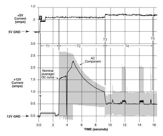
Figure 3. Typical Barracuda 4XL family drive +5 V and +12 V current profile
