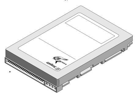
\*Model "N" version with 50 pin SCSI I/O connector
