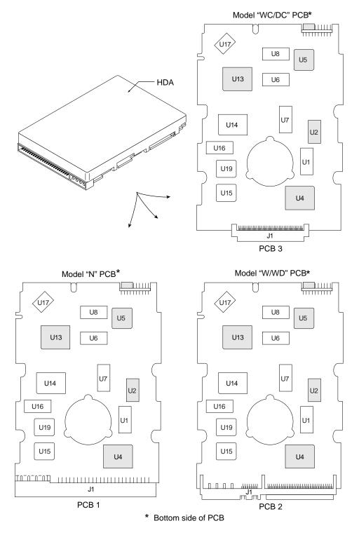
Figure 4. Locations of printed circuit board (PCB) components listed in Table 3
