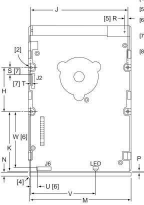
Figure 6. Mounting configuration dimensions for models "N"
